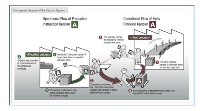
The Kanban system determines process production quantities, helping to facilitate just-in-time ordering systems and production. The system uses a labeled bin, card, or other device to indicate when more components are
